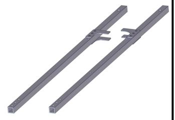
**<u>Step 16</u>**: Place a 90 Degree Gusset flush with both pieces. Mark and drill the two holes on the 32 inch 1x1 with a 3/16 inch bit.
