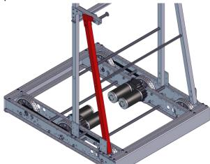
**Step 26**: Loosely secure the assembly to the cross Churro with the final 1/4-20 x 0.75 in. Thread Cutting Screw.
