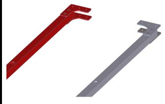
**Step 20**: Using the measurement and marking methods from before, on a 6.5 inch 1x1, notate a hole one inch from the end. Step drill this hole out to 5/8 inches.
