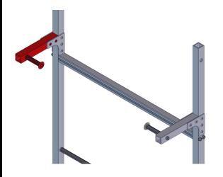
**Step 14**: This next step require some patience. Place the 32 inch 1x1 assembly onto the chassis, with the 90 Degree Gussets over the 6.5 inch 1x1.
